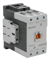
IronHorse IEC contactor, 85A, (3) N.O. power poles, (2) N.O./(2) N.C. auxiliary contacts, 480 VAC (60Hz) coil voltage.
