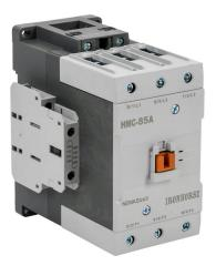
IronHorse IEC contactor, 85A, (3) N.O. power poles, (2) N.O./(2) N.C. auxiliary contacts, 230 VAC (50/60Hz) coil voltage.
