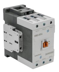
IronHorse IEC contactor, 85A, (3) N.O. power poles, (2) N.O./(2) N.C. auxiliary contacts, 24 VAC (50/60Hz) coil voltage.
