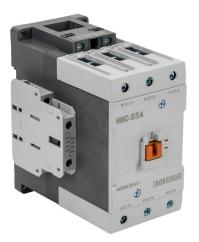
IronHorse IEC contactor, 85A, (3) N.O. power poles, (2) N.O./(2) N.C. auxiliary contacts, 120 VAC (50/60Hz) coil voltage.
