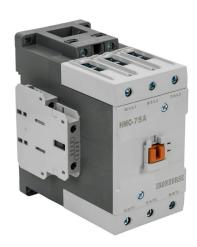
IronHorse IEC contactor, 75A, (3) N.O. power poles, (2) N.O./(2) N.C. auxiliary contacts, 24 VAC (50/60Hz) coil voltage.
