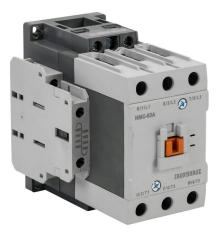
IronHorse IEC contactor, 65A, (3) N.O. power poles, (2) N.O./(2) N.C. auxiliary contacts, 480 VAC (60Hz) coil voltage.
