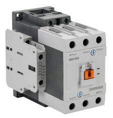
IronHorse IEC contactor, 65A, (3) N.O. power poles, (2) N.O./(2) N.C. auxiliary contacts, 24 VAC (50/60Hz) coil voltage.
