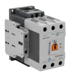
IronHorse IEC contactor, 50A, (3) N.O. power poles, (2) N.O./(2) N.C. auxiliary contacts, 480 VAC (60Hz) coil voltage.
