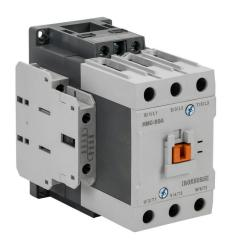
IronHorse IEC contactor, 50A, (3) N.O. power poles, (2) N.O./(2) N.C. auxiliary contacts, 24 VAC (50/60Hz) coil voltage.
