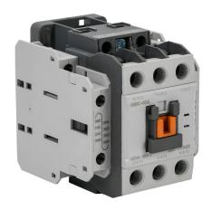
IronHorse IEC contactor, 40A, (3) N.O. power poles, (2) N.O./(2) N.C. auxiliary contacts, 480 VAC (60Hz) coil voltage.
