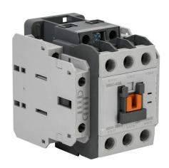
IronHorse IEC contactor, 40A, (3) N.O. power poles, (2) N.O./(2) N.C. auxiliary contacts, 230 VAC (50/60Hz) coil voltage.
