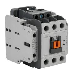
IronHorse IEC contactor, 40A, (3) N.O. power poles, (2) N.O./(2) N.C. auxiliary contacts, 24 VAC (50/60Hz) coil voltage.
