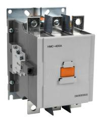
IronHorse IEC contactor, 400A, (3) N.O. power poles, (2) N.O./(2) N.C. auxiliary contacts, 100-240 VAC (50/60Hz)/100-200 VDC coil voltage, low consumption electronic.
