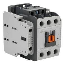
IronHorse IEC contactor, 32A, (3) N.O. power poles, (2) N.O./(2) N.C. auxiliary contacts, 480 VAC (60Hz) coil voltage.
