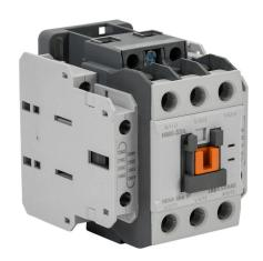
IronHorse IEC contactor, 32A, (3) N.O. power poles, (2) N.O./(2) N.C. auxiliary contacts, 230 VAC (50/60Hz) coil voltage.
