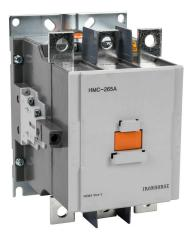
IronHorse IEC contactor, 265A, (3) N.O. power poles, (2) N.O./(2) N.C. auxiliary contacts, 100-240 VAC (50/60Hz)/100-200 VDC coil voltage, low consumption electronic.
