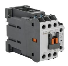
IronHorse IEC contactor, 22A, (3) N.O. power poles, (1) N.O./(1) N.C. auxiliary contacts, 24 VDC coil voltage.
