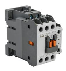
IronHorse IEC contactor, 22A, (3) N.O. power poles, (1) N.O./(1) N.C. auxiliary contacts, 230 VAC (50/60Hz) coil voltage.
