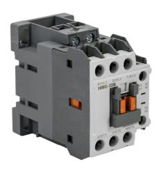
IronHorse IEC contactor, 22A, (3) N.O. power poles, (1) N.O./(1) N.C. auxiliary contacts, 24 VAC (50/60Hz) coil voltage.
