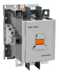
IronHorse IEC contactor, 225A, (3) N.O. power poles, (2) N.O./(2) N.C. auxiliary contacts, 100-240 VAC (50/60Hz)/100-200 VDC coil voltage, low consumption electronic.
