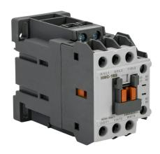
IronHorse IEC contactor, 18A, (3) N.O. power poles, (1) N.O./(1) N.C. auxiliary contacts, 24 VDC coil voltage.
