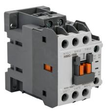
IronHorse IEC contactor, 18A, (3) N.O. power poles, (1) N.O./(1) N.C. auxiliary contacts, 24 VAC (50/60Hz) coil voltage.
