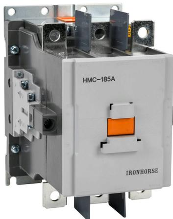
IronHorse IEC contactor, 185A, (3) N.O. power poles, (2) N.O./ (2) N.C. auxiliary contacts, 24-25VAC (50/60Hz)/24 VDC coil voltage, low consumption electronic.
