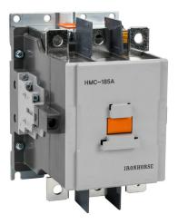
IronHorse IEC contactor, 185A, (3) N.O. power poles, (2) N.O./(2) N.C. auxiliary contacts, 100-240 VAC (50/60Hz)/100-200 VDC coil voltage, low consumption electronic.
