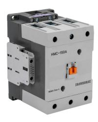
IronHorse IEC contactor, 150A, (3) N.O. power poles, (2) N.O./(2) N.C. auxiliary contacts, 24-48VAC (50/60Hz)/24-48 VDC coil voltage, low consumption electronic.
