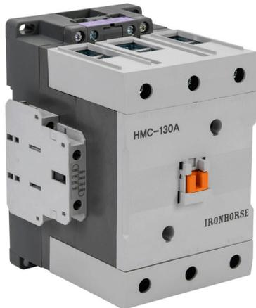
IronHorse IEC contactor, 130A, (3) N.O. power poles, (2) N.O./ (2) N.C. auxiliary contacts, 24-48VAC (50/60Hz)/24-48 VDC coil voltage, low consumption electronic.
