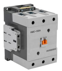
IronHorse IEC contactor, 130A, (3) N.O. power poles, (2) N.O./(2) N.C. auxiliary contacts, 100-240 VAC (50/60Hz)/100-200 VDC coil voltage, low consumption electronic.
