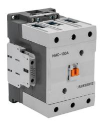
IronHorse IEC contactor, 130A, (3) N.O. power poles, (2) N.O./(2) N.C. auxiliary contacts, 24 VDC coil voltage.
