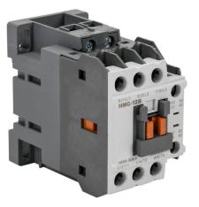
IronHorse IEC contactor, 12A, (3) N.O. power poles, (1) N.O./(1) N.C. auxiliary contacts, 480 VAC (60Hz) coil voltage.
