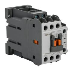
IronHorse IEC contactor, 12A, (3) N.O. power poles, (1) N.O./(1) N.C. auxiliary contacts, 24 VDC coil voltage.
