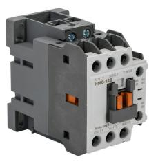
IronHorse IEC contactor, 12A, (3) N.O. power poles, (1) N.O./(1) N.C. auxiliary contacts, 230 VAC (50/60Hz) coil voltage.
