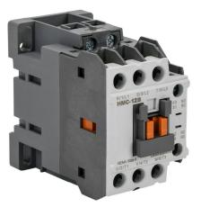
IronHorse IEC contactor, 12A, (3) N.O. power poles, (1) N.O./(1) N.C. auxiliary contacts, 120 VAC (50/60Hz) coil voltage.
