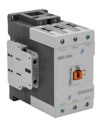
IronHorse IEC contactor, 100A, (3) N.O. power poles, (2) N.O./(2) N.C. auxiliary contacts, 24 VAC (50/60Hz) coil voltage.
