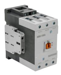
IronHorse IEC contactor, 100A, (3) N.O. power poles, (2) N.O./(2) N.C. auxiliary contacts, 120 VAC (50/60Hz) coil voltage.
