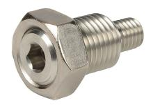
NITRA cylinder male adapter, M14  $\times$  1.5 thread, stainless steel. For use with 40mm H-series cylinders. Hex nut included.
