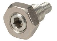
NITRA cylinder male adapter, M10 X 1.25 thread, stainless steel. For use with 25mm H-series cylinders. Hex nut included.
