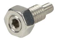
NITRA cylinder male adapter, M5 x 0.8 thread, stainless steel. For use with 12mm H-series cylinders. Hex nut included.
