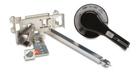
Eaton rotary handle, pistol, black, external front mount, 2-position, lockable in OFF only, defeatable, NEMA 4/4X. For use with AutomationDirect (Eaton) 600A frame MCCBs. 24in shaft and operator included.
