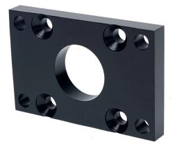
Peninsular flange mount plate, steel. For use with 4in bore x 2in rod hydraulic NFPA cylinders. Mounting hardware included.
