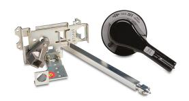
Eaton rotary handle, pistol, black, external front mount, 2-position, lockable in OFF only, defeatable, NEMA 4/4X. For use with AutomationDirect (Eaton) 400A frame MCCBs. 24in shaft and operator included.
