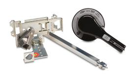
Eaton rotary handle, pistol, black, external front mount, 2-position, lockable in OFF only, defeatable, NEMA 4/4X. For use with AutomationDirect (Eaton) 225A frame MCCBs. 12in shaft and operator included.
