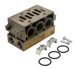
NITRA air manifold base, aluminum alloy, 145 psi (10 bar) maximum operating pressure, 3/8in female NPT outlet(s), side orientation. For use with ISO 5599/1 size 2 solenoid valves.
