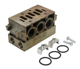
NITRA air manifold base, aluminum alloy, 145 psi (10 bar) maximum operating pressure, G3/8 female BSPP outlet(s), side orientation. For use with ISO 5599/1 size 2 solenoid valves.
