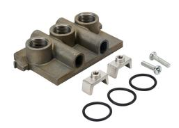
NITRA air manifold base, aluminum alloy, 145 psi (10 bar) maximum operating pressure, 1/2in female NPT inlet(s), 1/2in female NPT exhaust(s). For use with ISO 5599/1 size 2 manifolds.
