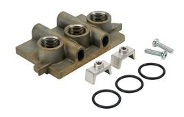
NITRA air manifold inlet, aluminum alloy, 145 psi (10 bar) maximum operating pressure, G1/2 female BSPP inlet(s), G1/2 female BSPP exhaust(s). For use with ISO 5599/1 size 2 manifolds.
