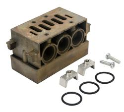
NITRA air manifold base, aluminum alloy, 145 psi (10 bar) maximum operating pressure, 3/8in female NPT outlet(s), bottom orientation. For use with ISO 5599/1 size 2 solenoid valves.
