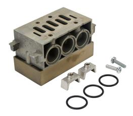
NITRA air manifold base, aluminum alloy, 145 psi (10 bar) maximum operating pressure, G3/8 female BSPP outlet(s), bottom orientation. For use with ISO 5599/1 size 2 solenoid valves.
