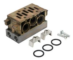
NITRA air manifold base, aluminum alloy, 145 psi (10 bar) maximum operating pressure, 1/4in female NPT outlet(s), side orientation. For use with ISO 5599/1 size 1 solenoid valves.
