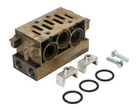
NITRA air manifold base, aluminum alloy, 145 psi (10 bar) maximum operating pressure, G1/4 female BSPP outlet(s), side orientation. For use with ISO 5599/1 size 1 solenoid valves.
