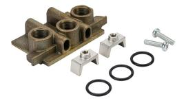
NITRA air manifold inlet, aluminum alloy, 145 psi (10 bar) maximum operating pressure, 3/8in female NPT inlet(s), 3/8in female NPT exhaust(s). For use with ISO 5599/1 size 1 manifolds.
